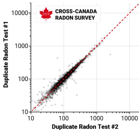
For this graph, the 'coefficient of determination' value ( $r^2$ ) is 0.97, which is considered an extremely strong indication of precision.
