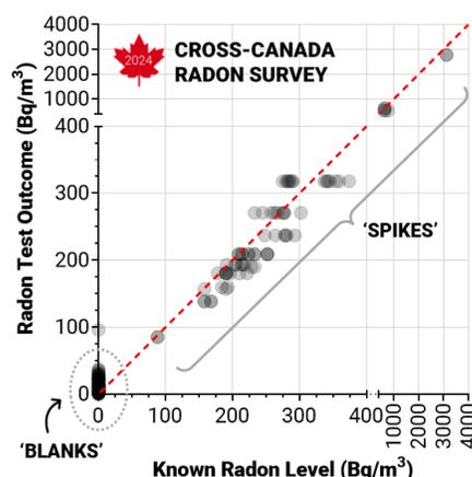
For this graph, the ‘coefficient of determination’ value ( $r^2$ ) is 0.995, which is considered an extremely strong indication of accuracy.
