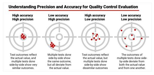
reliability of results in terms of **accuracy** and **precision**, which are explained in the graphic above. To illustrate quality controls used to assess accuracy and precision, data from radon tests conducted by the Evict Radon National Study team are shown in the examples below.
